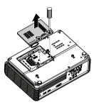
4. Loosen the two captive screws that secure the lamp.
