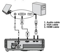
Many notebooks do not turn on their external video ports when connected to a projector. Usually a key combo like FN + F3 or CRT/LCD key turns the external display on/ off. Locate a function key labeled CRT/LCD or a function key with a monitor symbol on the notebook. Press FN and the labeled function key simultaneously. Refer to your notebook's documentation to find your notebook's key combination.
