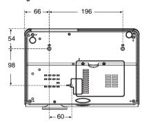
\* Ceiling Mount Screws: M4 x 14 (Max. L=14, Min. L=12)
